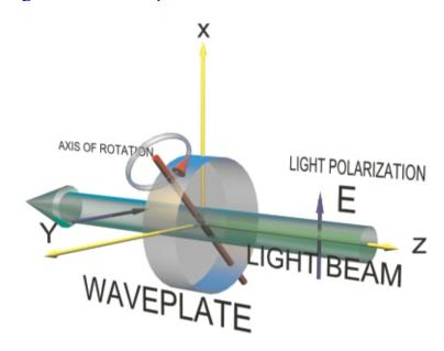
The required phase retardation is achieved by tilting the plates by 8° - 15°. This design is aimed at avoiding light reflection back to the laser system which in many cases results in complications.
