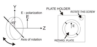
3. Rotate the screw, until the required retardation is achieved.
